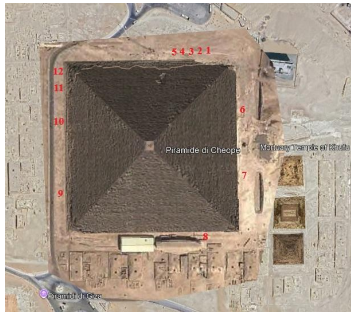
Fig. 6 The G1 pyramid of Akhet Khufu, with the points where I measured relative erosion marked in red (picture from Googleearth)
