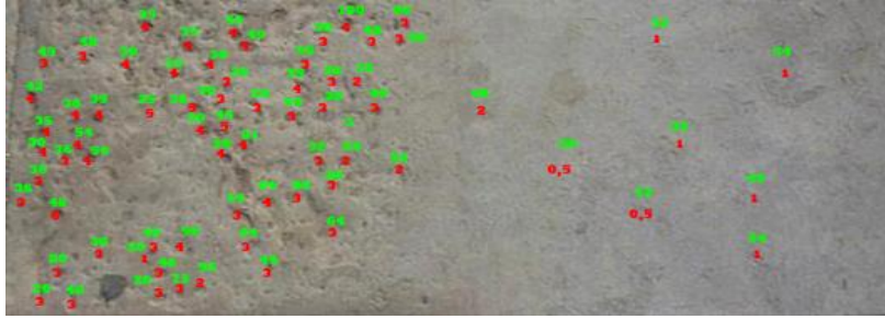
Fig. 8 Calculation of erosion (volume of holes) in point 2: on the right, the part of the limestone pavement exposed to erosive agents for approximately 675 years; on the left, the part exposed since the time of construction.
